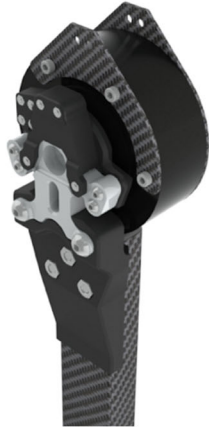
Fig S6. Experimental setup utilized to perform the engineering validation of the hip configuration. (A) Modified hip exoskeleton design incorporating a torque transducer. This modified design featured altered 3D printed components to link the motor to the carbon fiber upright while incorporating the torque sensor into these components. This version of the design was only used for the engineering validation work. (B) Image of benchtop testing setup. The motor-upright assembly was secured to a table via clamps and vices to prevent movement. The codebase was modified to include a new exoskeleton controller designed to apply step commands with user defined amplitudes, duration, and spacing (included as part of OpenExo's software). A series of open-loop step commands were sent to the motor while recording the measured torque.
